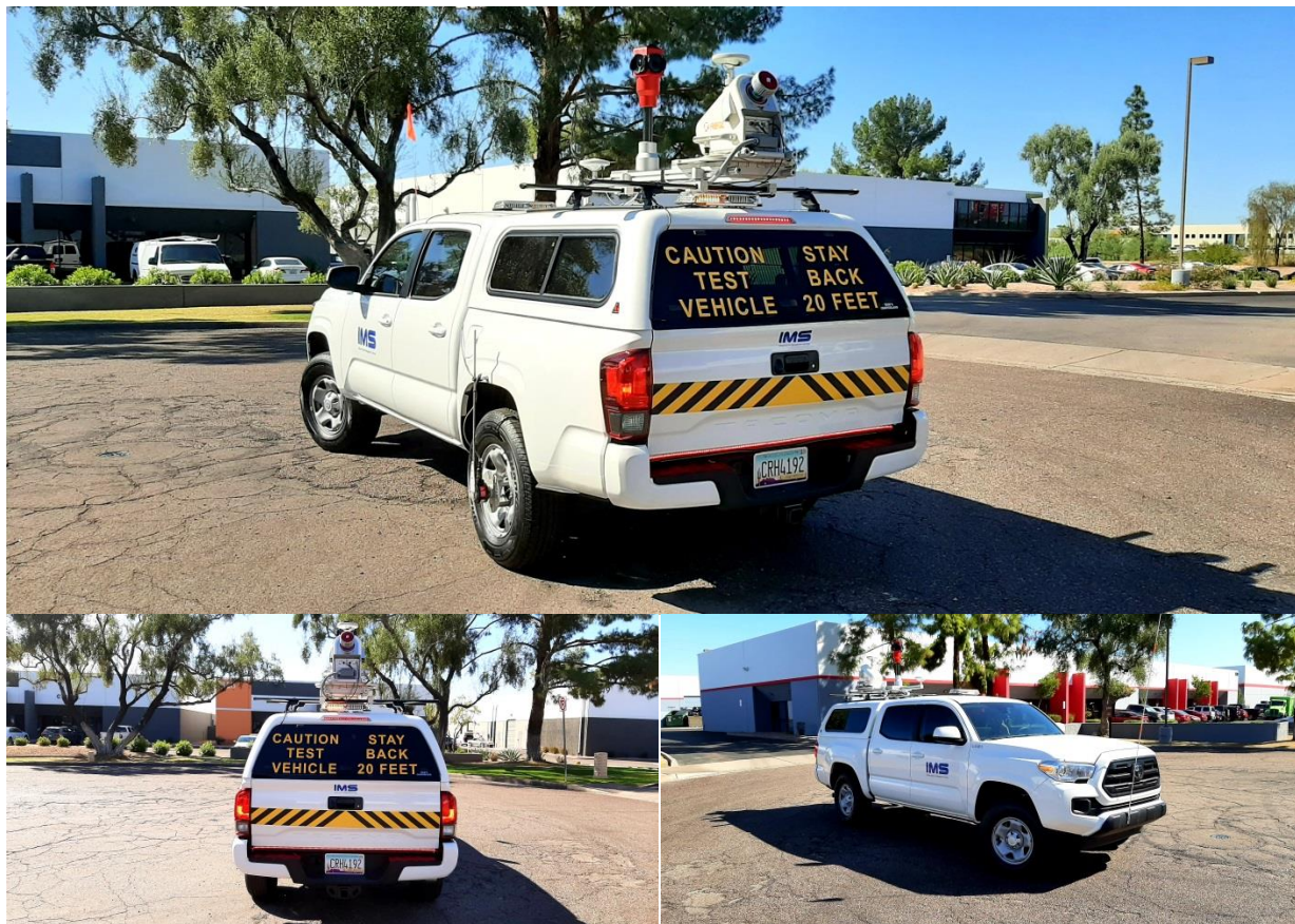
Figure 2 – LiDAR Survey Unit
